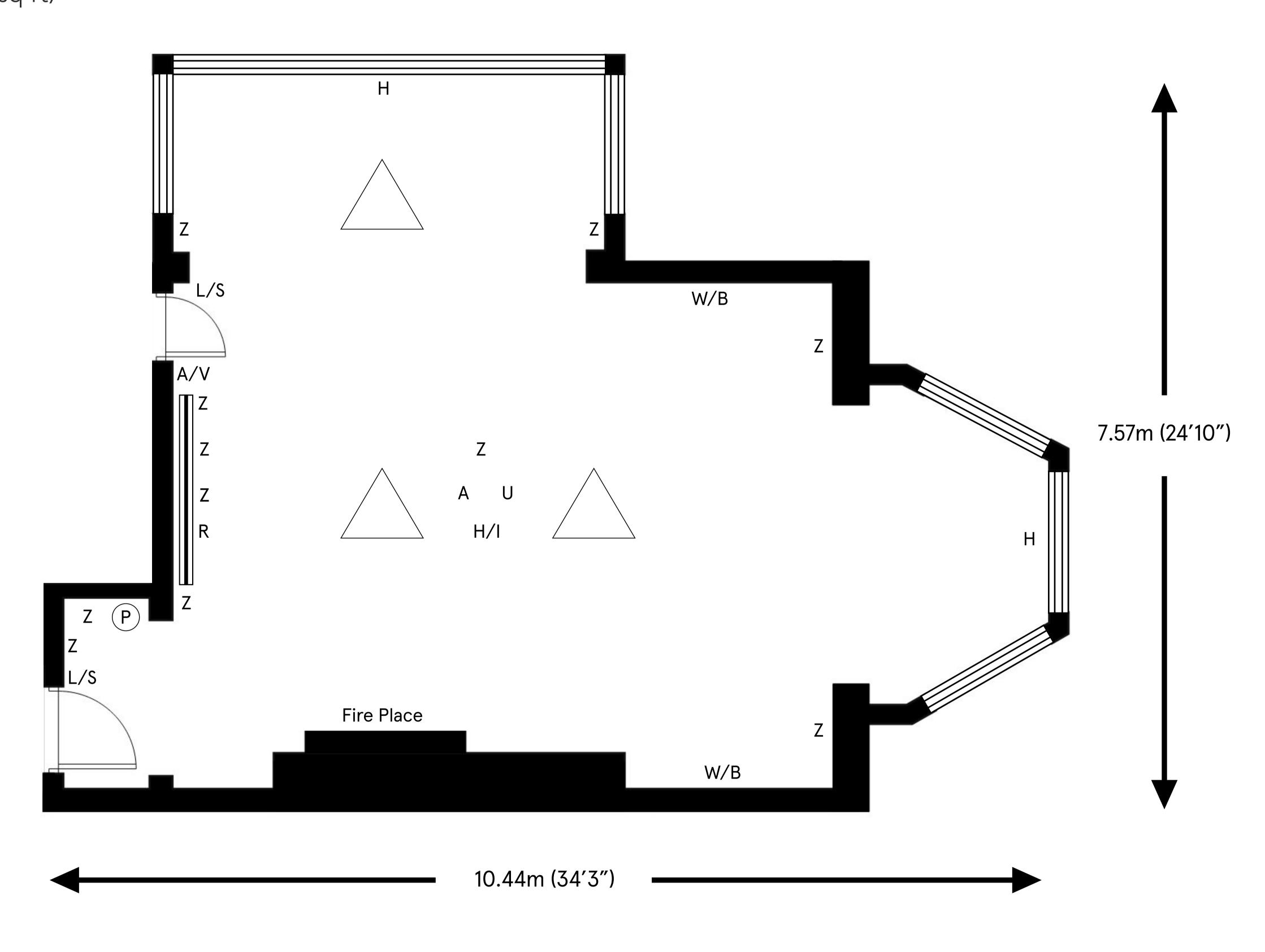
Key:Z13 Amp SocketsUUSBPPhone Line△ChandelierAAudio OutletsHHeaterL/SLight switchA/V A/V Switch BoardW/BWhite BoardH/IHDMI Input■Electric Screen
